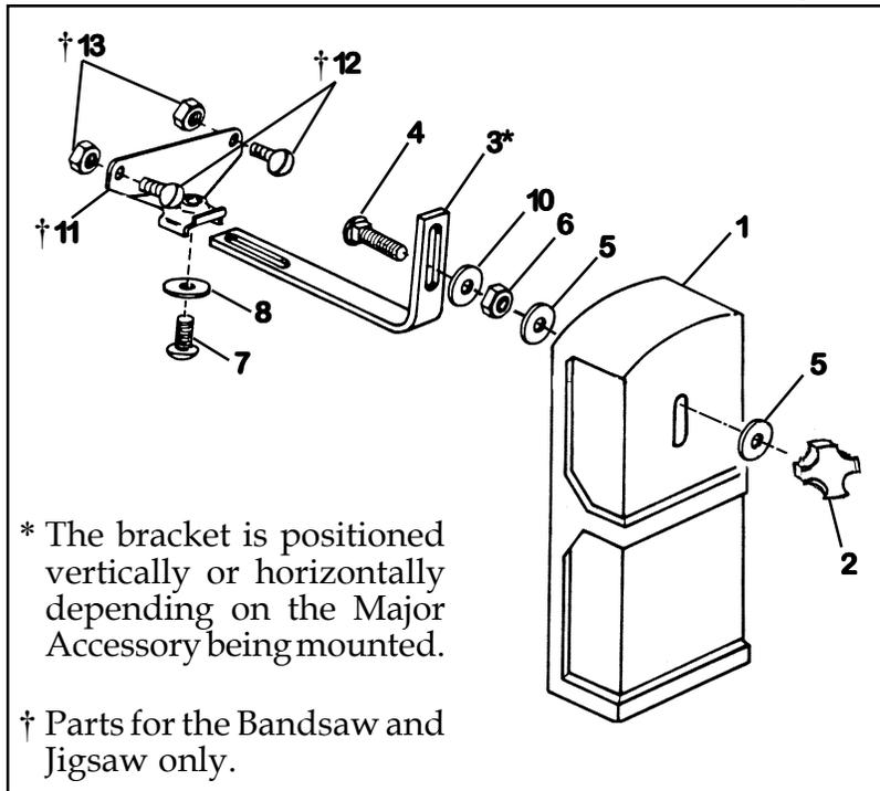
\* The bracket is positioned vertically or horizontally depending on the Major Accessory being mounted.
